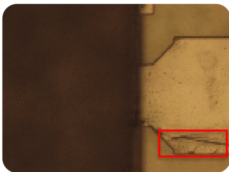
Failure/ crack (opt. Microscope)
